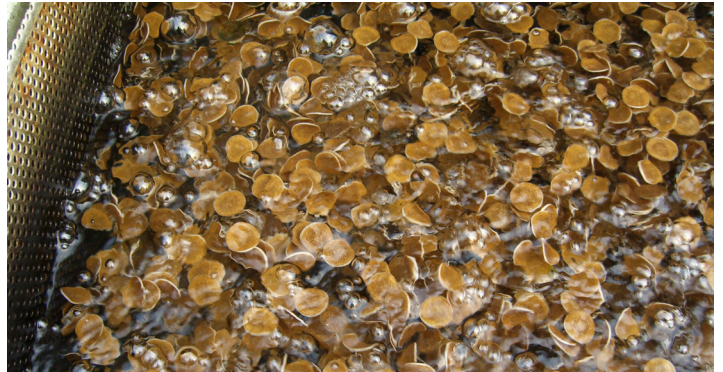
Nitrification by means of Mutag BioChip™ RAS process in a fish farm.
